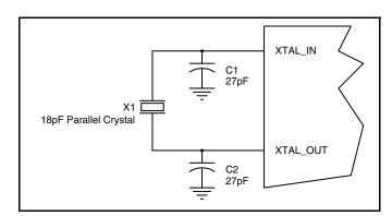
Figure 1. Crystal Input Interface
