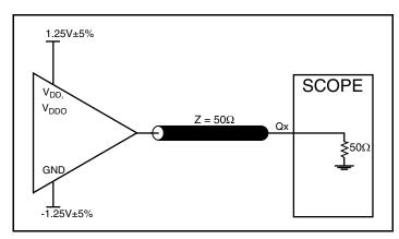
2.5V/2.5V Output Load AC Test Circuit
