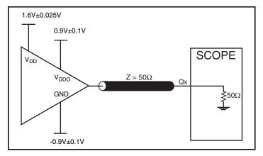
2.5V/1.8V Output Load AC Test Circuit
