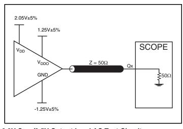
3.3V Core/2.5V Output Load AC Test Circuit
