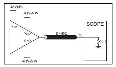
3.3V Core/1.8V Output Load AC Test Circuit
