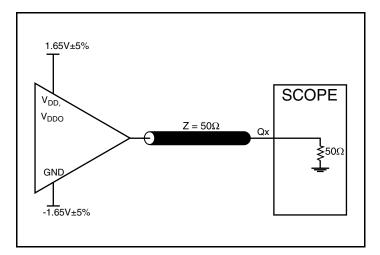
3.3 Core/3.3V Output Load AC Test Circuit
