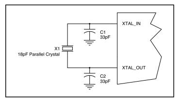
Figure 2. Crystal Input Interface
