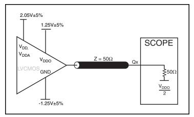
3.3V Core/2.5V Output Load AC Test Circuit
