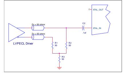
Figure 1B. General Diagram for LVPECL Driver to XTAL Input Interface
