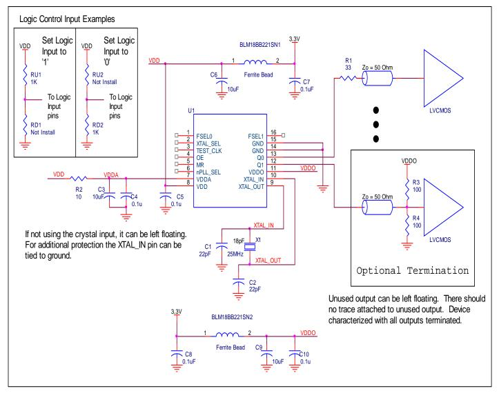
Figure 2. 840002-01 Application Schematic Example
