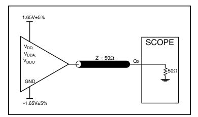
3.3V Core/3.3V Output Load AC Test Circuit
