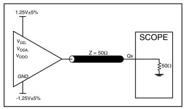
2.5V Core/2.5V Output Load AC Test Circuit
