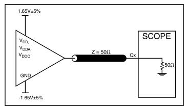
3.3V Core/3.3V Output Load AC Test Circuit
