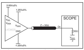
3.3V Core/2.5V Output Load AC Test Circuit
