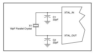
Figure 2. Crystal Input Interface
