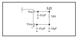
Figure 1. Power Supply Filtering
