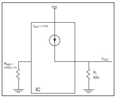
Figure 7. HCSL Driver Circuit and Termination
