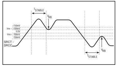
**Differential Measurement Points for Ringback**
