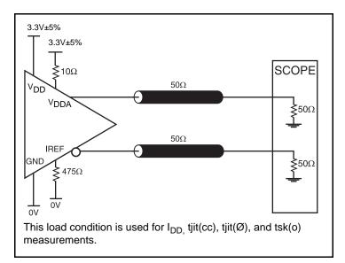
3.3V HCSL Output Load Test Circuit
