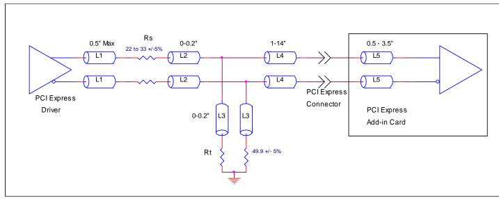
Figure 4A. Recommended Source Termination (where the driver and receiver will be on separate PCBs)
