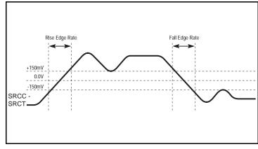
Differential Measurement Points for Rise/Fall Edge Rate
