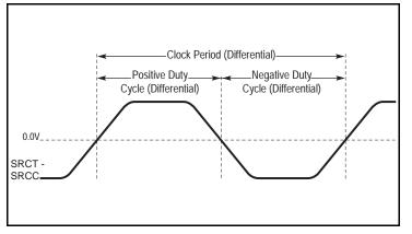
**Differential Measurement Points for Duty Cycle/Period**
