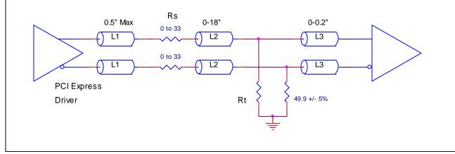
Figure 4B. Recommended Termination (where a point-to-point connection can be used)
