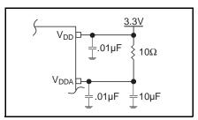
Figure 1. Power Supply Filtering
