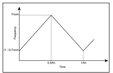
Figure 6A. Triangle Frequency Modulation
