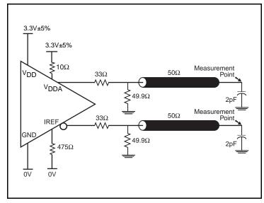
3.3V HCSL Output Load Test Circuit
