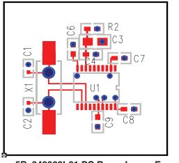
FIGURE 5B. 843002I-01 PC BOARD LAYOUT EXAMPLE
