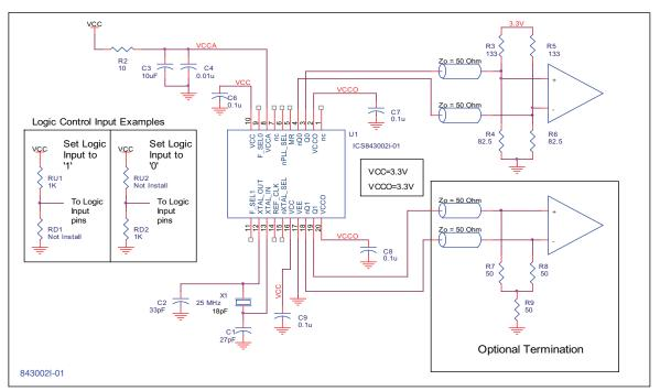
FIGURE 5A. 843002I-01 SCHEMATIC EXAMPLE
