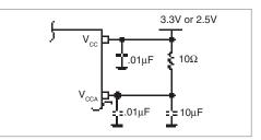
FIGURE 1. POWER SUPPLY FILTERING
