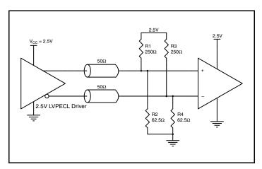
Figure 6A. 2.5V LVPECL Driver Termination Example
