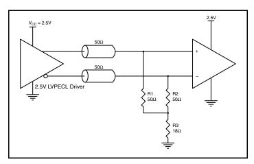
Figure 6B. 2.5V LVPECL Driver Termination Example
