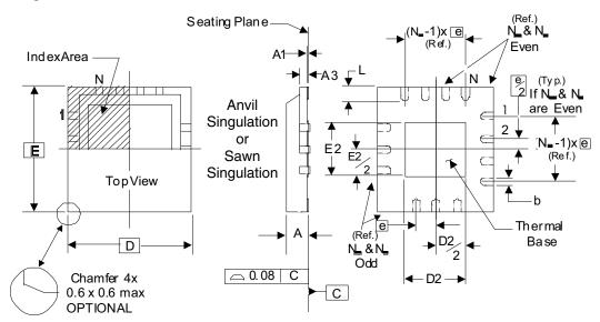
NOTE: The following package mechanical drawing is a generic drawing that applies to any pin count VFQFN package. This drawing is not intended to convey the actual pin count or pin layout of this device. The pin count and pinout are shown on the front page. The package dimensions are in Table 8 below.
