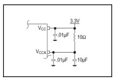
Figure 1. Power Supply Filtering
