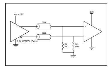
Figure 6C. 2.5V LVPECL Driver Termination Example
