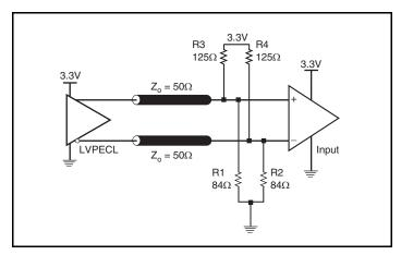
Figure 5B. 3.3V LVPECL Output Termination
