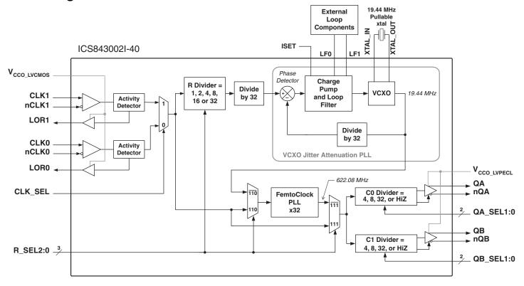
NOTE: 19.44MHz VCXO crystal shown is typical for SONET/SDH device applications.
