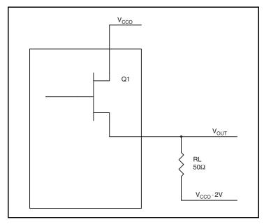
Figure 8. LVPECL Driver Circuit and Termination
