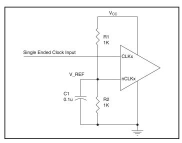
Figure 2. Single-Ended Signal Driving Differential Input
