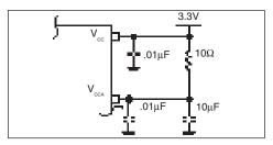
FIGURE 2. POWER SUPPLY FILTERING
