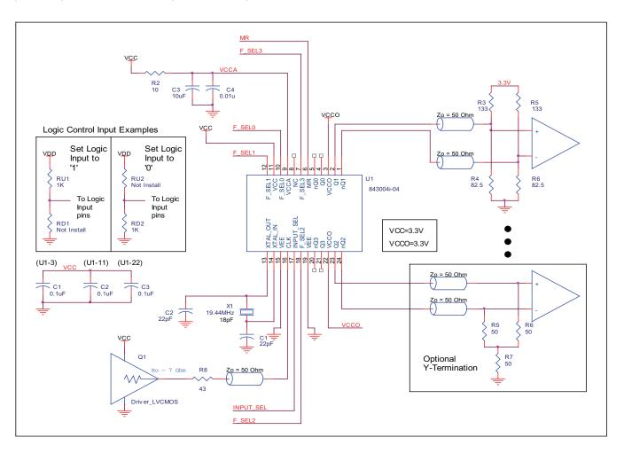
FIGURE 5. ICS844004I-04 SCHEMATIC EXAMPLE
