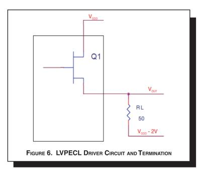
To calculate worst case power dissipation into the load, use the following equations which assume a 50 $\Omega$  load, and a termination voltage of V<sub>cc</sub>- 2V.
