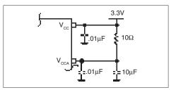
FIGURE 1. POWER SUPPLY FILTERING
