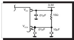
FIGURE 1. POWER SUPPLY FILTERING
