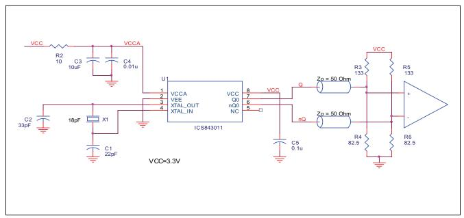
FIGURE 3A. 843011 SCHEMATIC EXAMPLE
