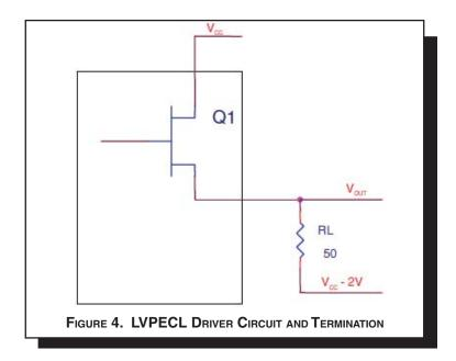
To calculate worst case power dissipation into the load, use the following equations which assume a  $50\Omega$  load, and a termination voltage of  $V_{cc}$ - 2V.
