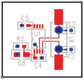
FIGURE 3B. 843011 PC BOARD LAYOUT EXAMPLE
