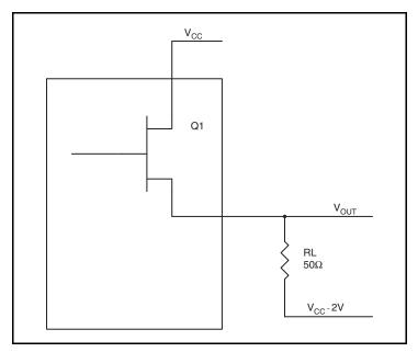
Figure 6. LVPECL Driver Circuit and Termination
