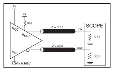
3.3V LVPECL Output Load AC Test Circuit
