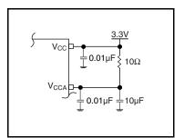
Figure 1. Power Supply Filtering
