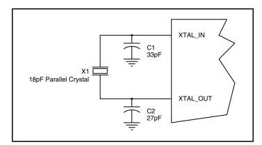
Figure 2. Crystal Input Interface
