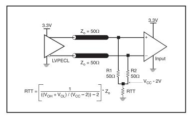
Figure 4A. 3.3V LVPECL Output Termination
