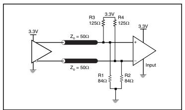
Figure 4B. 3.3V LVPECL Output Termination
