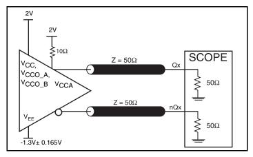
3.3V LVPECL Output Load AC Test Circuit
