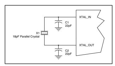
Figure 2. Crystal Input Interface
