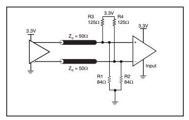
Figure 4B. 3.3V LVPECL Output Termination
