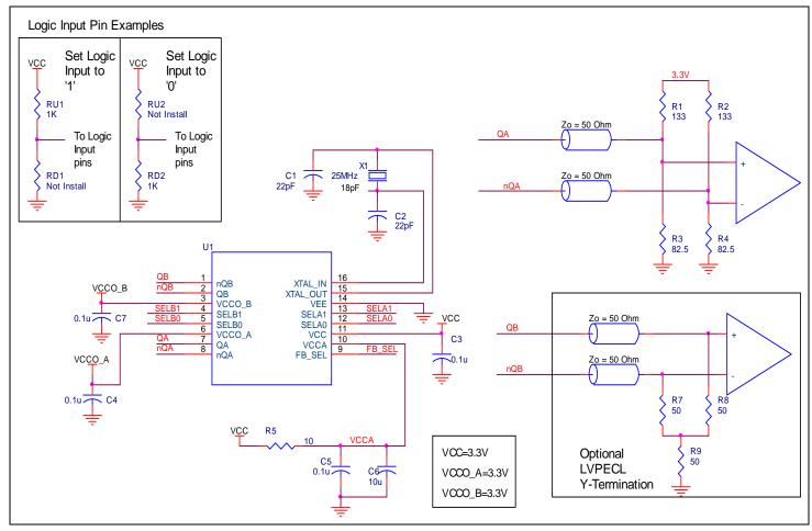
Figure 5. 843252 Schematic Example
