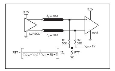
Figure 4A. 3.3V LVPECL Output Termination
