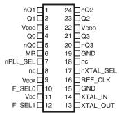
ICS844004I-01 24-Lead TSSOP 4.4mm x 7.8mm x 0.92mm package body **G** Package **Top View**
