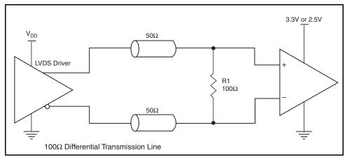
Figure 4. Typical LVDS Driver Termination
