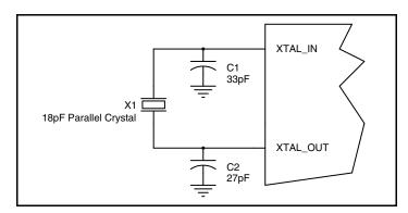
Figure 2. Crystal Input Interface
