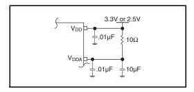
Figure 1. Power Supply Filtering
