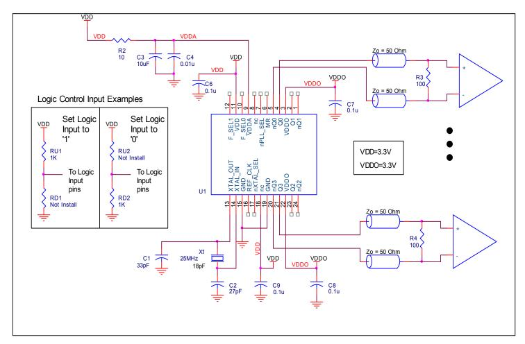
Figure 5. ICS844004I-01 Schematic Layout Example
