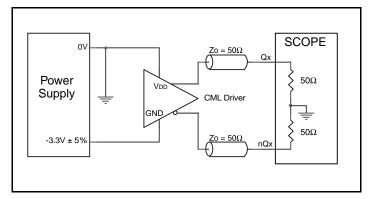
3.3V CML Output Load AC Test Circuit
