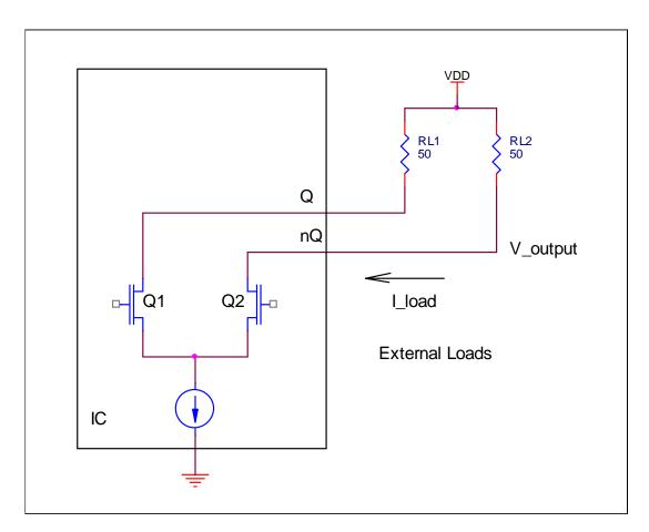
Figure 6. CML Driver Circuit and Termination
