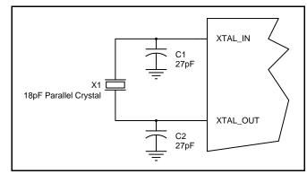
Figure 2. Crystal Input Interface
