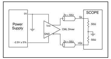
2.5V CML Output Load AC Test Circuit
