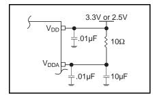
Figure 1. Power Supply Filtering
