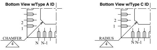
There are 2 methods of indicating pin 1 corner at the back of the VFQFN package:
