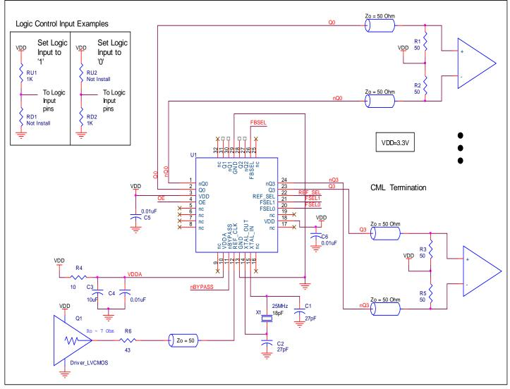
Figure 5. 845254 Schematic Layout Example
