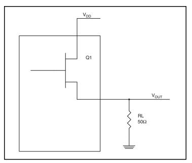
Figure 4. LVHSTL Driver Circuit and Termination
