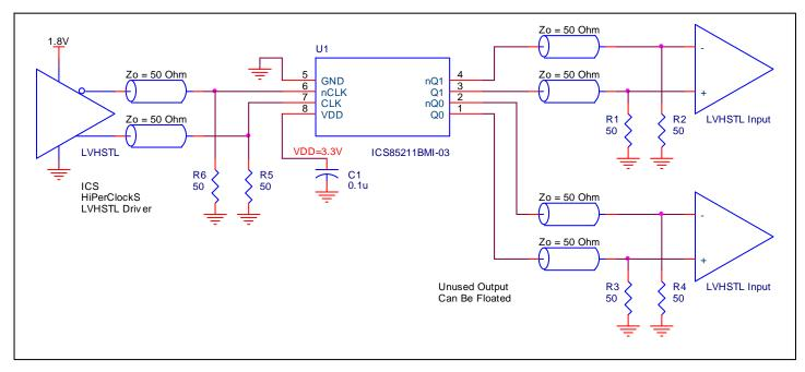
Figure 3. 85211BI-03 LVHSTL Buffer Schematic Example
