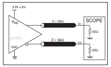
**Output Load AC Test Circuit**
