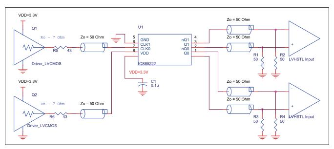
FIGURE 1. 85222 LVHSTL BUFFER SCHEMATIC EXAMPLE
