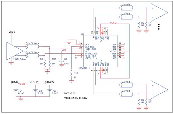
FIGURE 4. 8529111 HSTL BUFFER SCHEMATIC EXAMPLE
