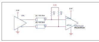
FIGURE 3A. PECL\_CLK/nPECL\_CLK INPUT DRIVEN BY A CML DRIVER
