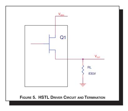
To calculate worst case power dissipation into the load, use the following equations which assume a  $50\Omega$  load.
