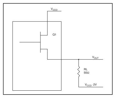
Figure 4. LVPECL Driver Circuit and Termination
