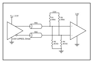
Figure 3A. 2.5V LVPECL Driver Termination Example
