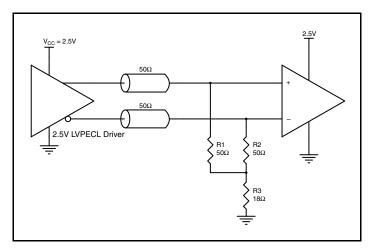
Figure 3B. 2.5V LVPECL Driver Termination Example
