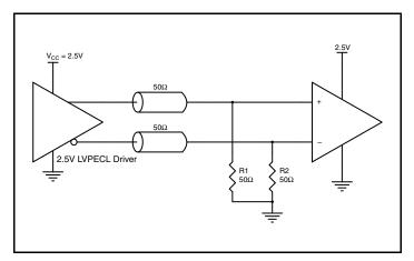
Figure 3C. 2.5V LVPECL Driver Termination Example
