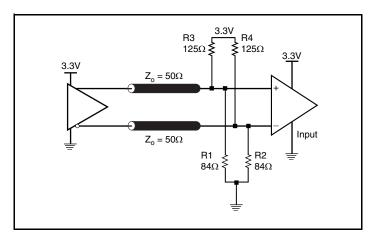
Figure 4B. 3.3V LVPECL Output Termination
