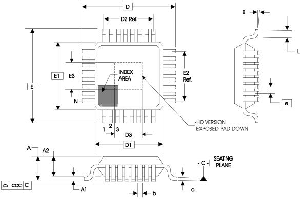
Table 8. Package Dimensions 48 Lead TQFP, E-Pad
