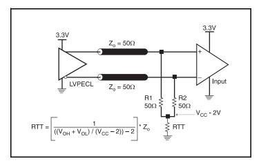
Figure 4A. 3.3V LVPECL Output Termination
