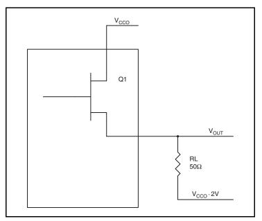
Figure 5. LVPECL Driver Circuit and Termination
