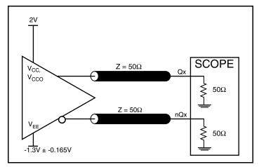
LVPECL Output Load AC Test Circuit
