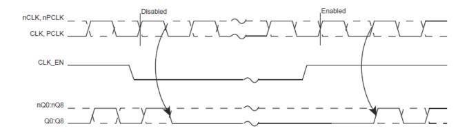
FIGURE 1. CLK\_EN TIMING DIAGRAM
