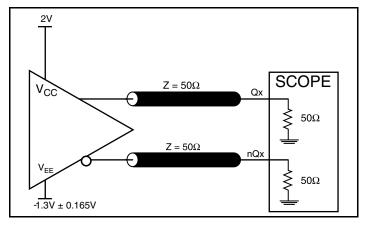
3.3V LVPECL Output Load AC Test Circuit
