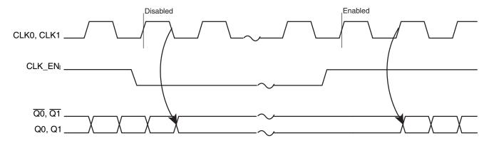
Figure 1. CLK\_EN Timing Diagram
