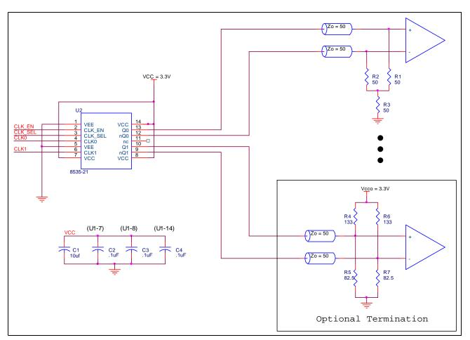
Figure 3. 8535-21 LVPECL Buffer Schematic Example
