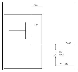
Figure 4. LVPECL Driver Circuit and Termination
