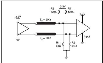
Figure 2B. 3.3V LVPECL Output Termination
