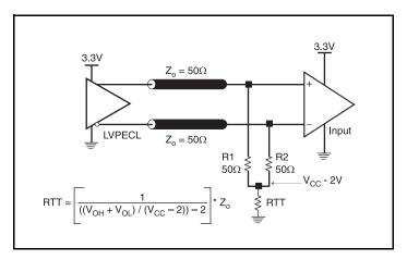
Figure 2A. 3.3V LVPECL Output Termination
