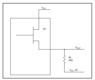
Figure 4. LVPECL Driver Circuit and Termination
