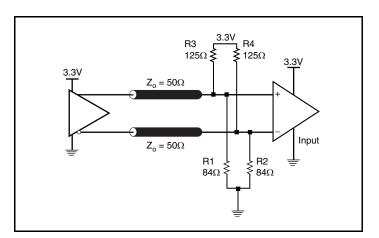
Figure 3B. 3.3V LVPECL Output Termination
