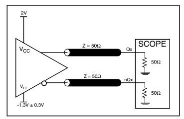
LVPECL Output Load AC Test Circuit
