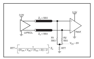
Figure 3A. 3.3V LVPECL Output Termination
