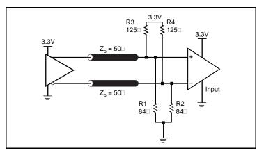
Figure 4B. 3.3V LVPECL Output Termination
