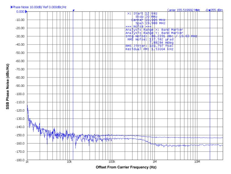
As with most timing specifications, phase noise measurements have issues. The primary issue relates to the limitations of the equipment. Often the noise floor of the equipment is higher than the noise floor of the device. This is illustrated above. The device meets the noise floor of what is shown, but can actually be lower. The phase noise is dependent on the input source and measurement equipment.
