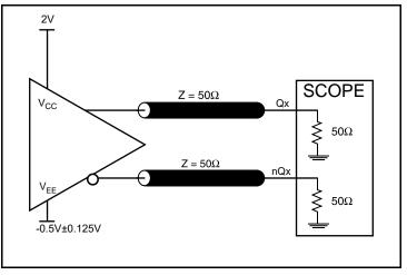
2.5V Output Load Test Circuit
