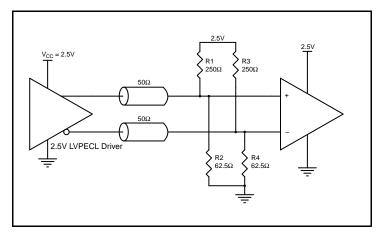
Figure 5A. 2.5V LVPECL Driver Termination Example
