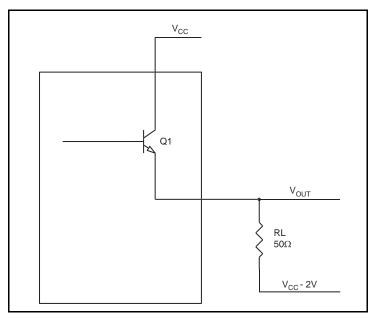
Figure 4. LVPECL Driver Circuit and Termination
