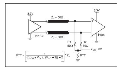
Figure 4A. 3.3V LVPECL Output Termination
