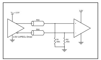
Figure 5C. 2.5V LVPECL Driver Termination Example
