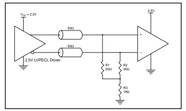
Figure 5B. 2.5V LVPECL Driver Termination Example
