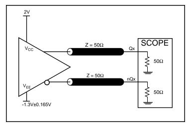
3.3V Output Load Test Circuit
