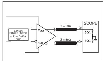
3.3V LVDS Output Load AC Test Circuit
