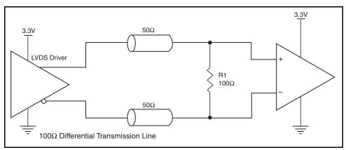
Figure 1. Typical LVDS Driver Termination
