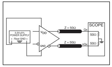
3.3V LVDS Output Load AC Test Circuit
