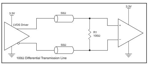
Figure 1. Typical LVDS Driver Termination
