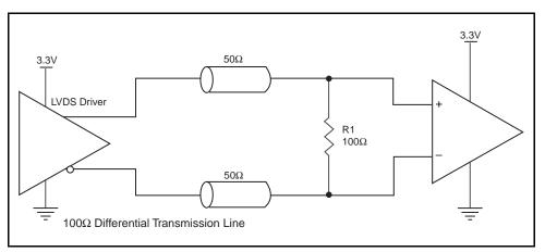
Figure 2. Typical LVDS Driver Termination
