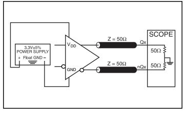
3.3V LVDS Output Load AC Test Circuit
