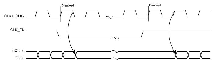
Figure 1. CLK\_EN Timing Diagram
