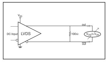
**Differential Output Voltage Setup**
