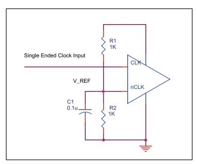
FIGURE 1. SINGLE ENDED SIGNAL DRIVING DIFFERENTIAL INPUT
