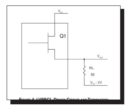
To calculate worst case power dissipation into the load, use the following equations which assume a  $50\Omega$  load, and a termination voltage of  $V_{cc}$ - 2V.
