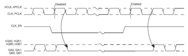
FIGURE 1 - CLK\_EN TIMING DIAGRAM
