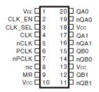
8737I-11 20-Lead TSSOP 6.50mm x 4.40mm x 0.92 package body G Package Top View
