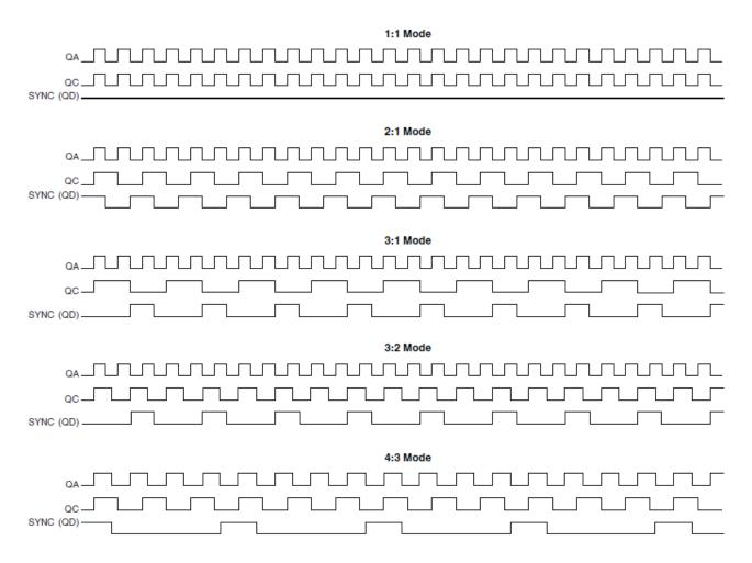
FIGURE 1. TIMING DIAGRAMS
