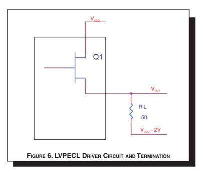
To calculate worst case power dissipation into the load, use the following equations which assume a 50 $\Omega$  load, and a termination voltage of V<sub>cco</sub>- 2V.
