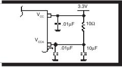
FIGURE 2. POWER SUPPLY FILTERING
