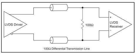
**Figure 4. Typical LVDS Driver Termination**
