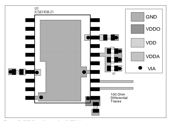
Figure 6B. PCB Board Layout for 8745BI-21
