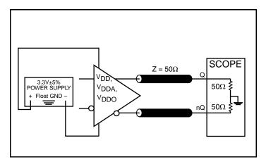
3.3V LVDS Output Load AC Test Circuit
