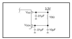
Figure 1. Power Supply Filtering
