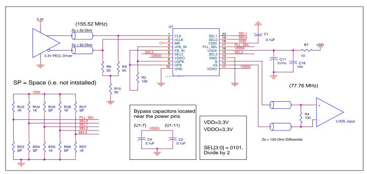
Figure 6A. 8745BI-21 LVDS Zero Delay Buffer Schematic Example
