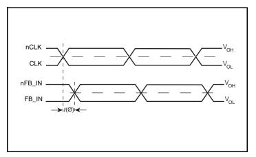
**Phase Jitter and Static Phase Offset**
