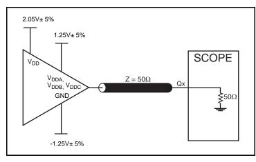
3.3V Core/2.5V Output Load AC Test Circuit
