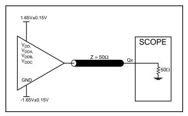
3.3V Core/3.3V Output Load AC Test Circuit
