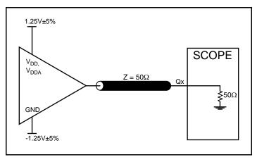
2.5V Output Load AC Test Circuit
