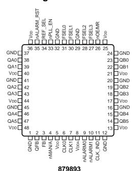
48-Lead LQFP 7mm x 7mm x 1.4mm package body Y Package Top View
