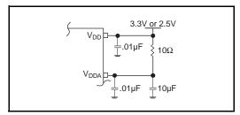
Figure 1. Power Supply Filtering
