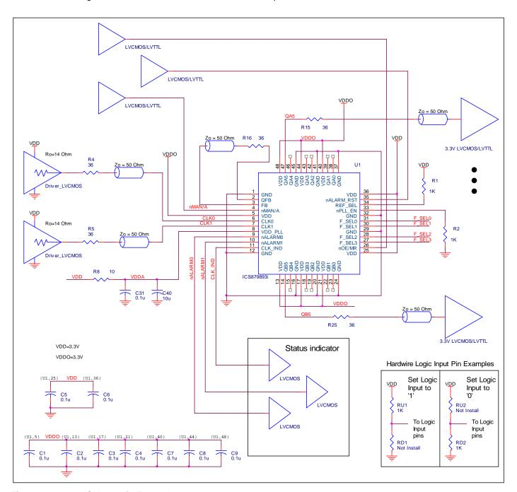
Figure 2. 879893 Schematic Example
