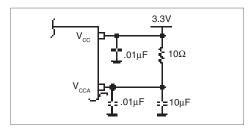
FIGURE 1. POWER SUPPLY FILTERING
