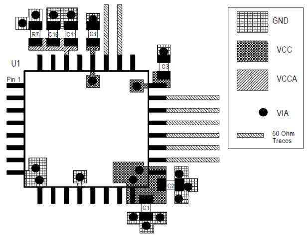
FIGURE 5B. PCB BOARD LAYOUT FOR 87993I
