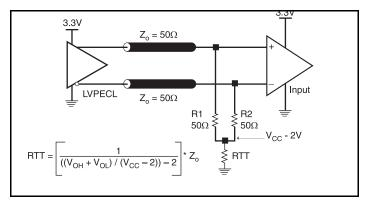
Figure 3A. 3.3V LVPECL Output Termination
