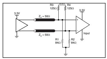
Figure 3B. 3.3V LVPECL Output Termination
