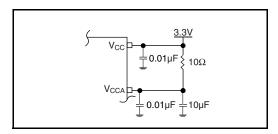
Figure 2. Power Supply Filtering
