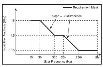
**Jitter Tolerance Specification**
