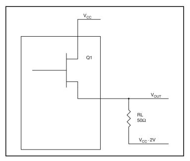
Figure 4. LVPECL Driver Circuit and Termination
