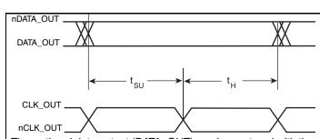
The re-timed data output (DATA\_OUT) can be captured with the rising edge of the clock output signal (CLOCK\_OUT). DATA\_OUT is valid the specified setup time before the rising CLK\_OUT signal and remains valid the specified hold time after the rising edge of the CLK\_OUT signal.
