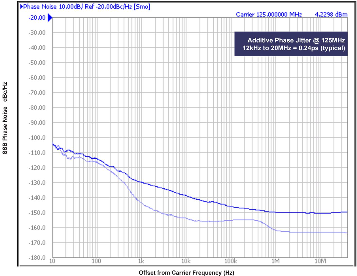
As with most timing specifications, phase noise measurements has issues relating to the limitations of the equipment. Often the noise floor of the equipment is higher than the noise floor of the device. The phase noise is dependent on the input source and measurement
