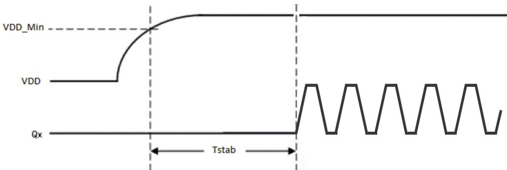
**Figure 1. Stabilization Time (T<sub>stab</sub>)**
