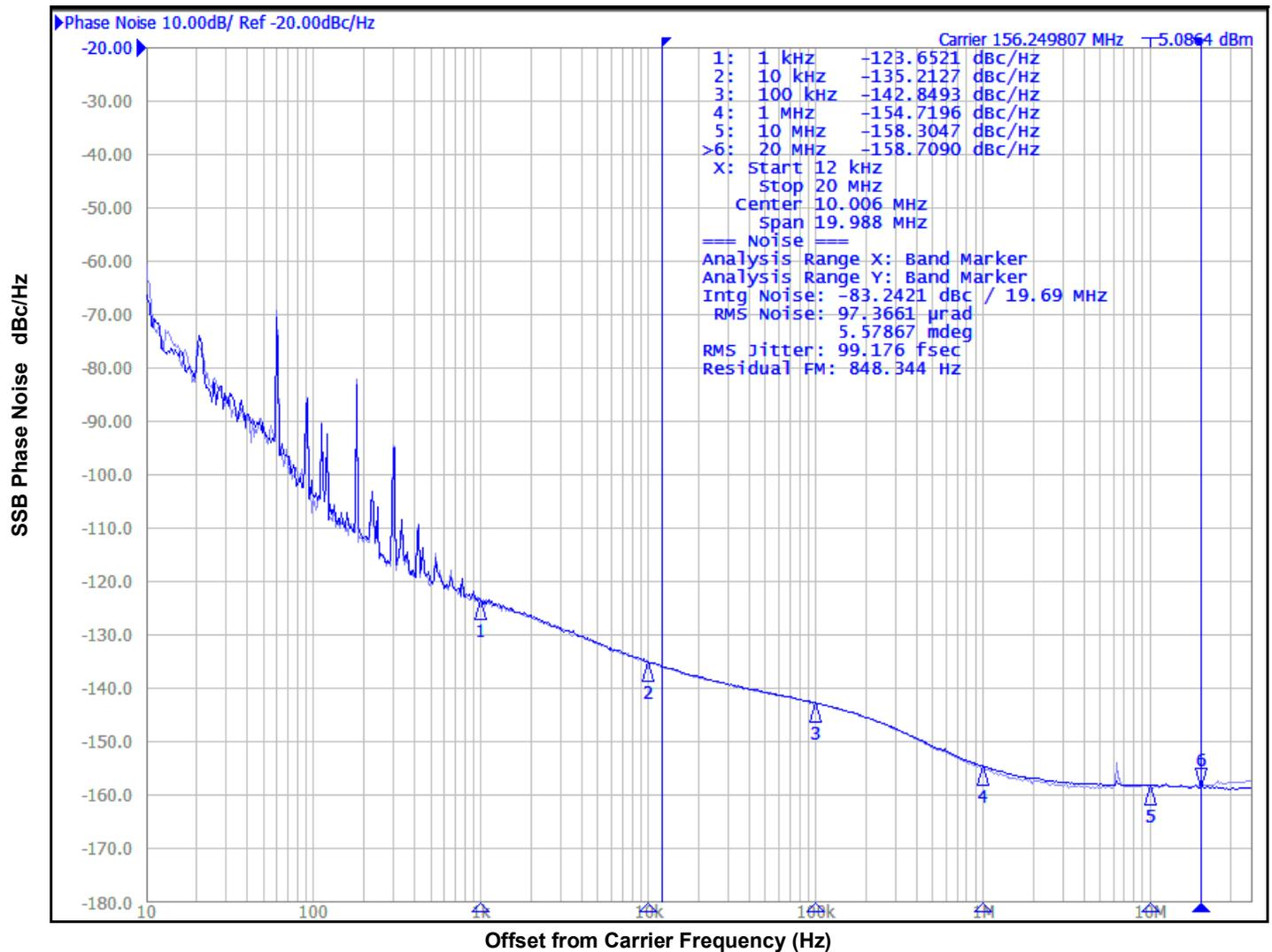
As with most timing specifications, phase noise measurements have issues relating to the limitations of the measurement equipment. The noise floor of the equipment can be higher or lower than the noise floor of the device. Additive phase noise is dependent on both the noise floor of the input source and measurement equipment.
