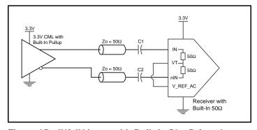
Figure 2D. IN/nIN Input with Built-In 50 $\Omega$  Driven by a CML Driver with Built-In 50 $\Omega$  Pullup
