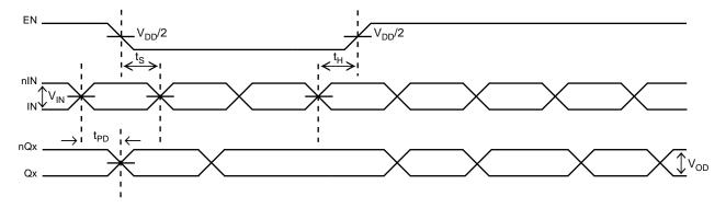
Figure 1. EN Timing Diagram
