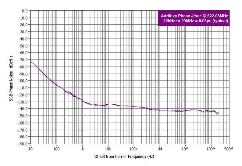
As with most timing specifications, phase noise measurements has issues relating to the limitations of the equipment. Often the noise floor of the equipment is higher than the noise floor of the device. This is illustrated above. The device meets the noise floor of what is shown, but can actually be lower. The phase noise is dependent on the input source and measurement equipment.
