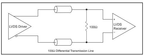
Figure 4. Typical LVDS Driver Termination
