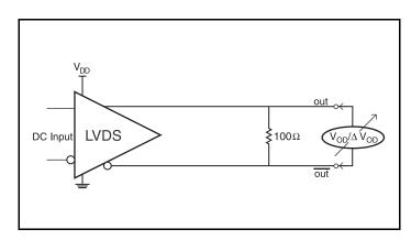
**Differential Output Voltage Setup**
