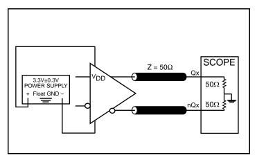
**LVDS Output Load AC Test Circuit**
