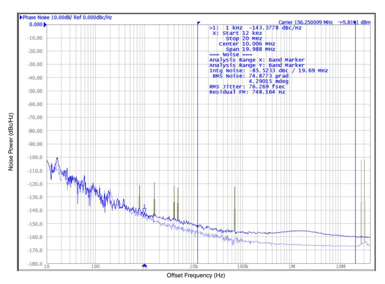
As with most timing specifications, phase noise measurements have issues relating to the limitations of the measurement equipment. The noise floor of the equipment can be higher or lower than the noise floor of the device. Additive phase noise is dependent on both the noise floor of the input source and measurement equipment. Additive phase jitter was measured with a Wenzel 156.25MHz oscillator as the input source.
