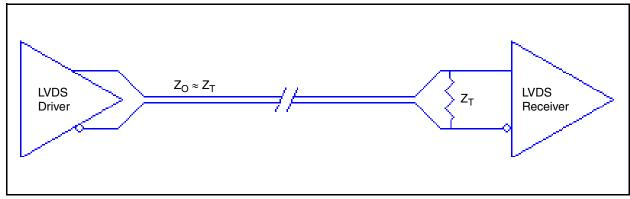
Figure 3A. Standard LVDS Termination
