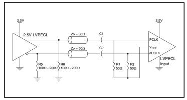
Figure 2D. PCLK/nPCLK Input Driven by a 2.5V LVPECL Driver AC Couple with V<sub>REF</sub> bias
