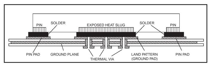
Figure 4. P.C. Assembly for Exposed Pad Thermal Release Path - Side View (drawing not to scale)
