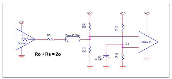
Figure 1B. Alternative DC Coupling a Single LVCMOS Input to the 8SLVP1212
