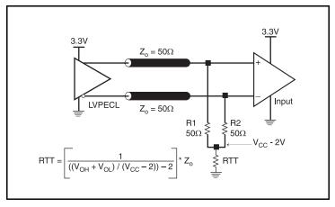
Figure 5A. 3.3V LVPECL Output Termination
