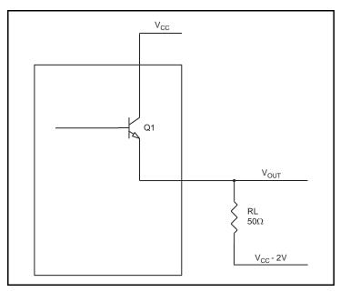
Figure 8. LVPECL Driver Circuit and Termination
