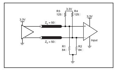
Figure 5B. 3.3V LVPECL Output Termination
