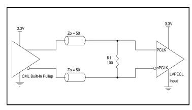
Figure 2B. PCLK/nPCLK Input Driven by a Built-In Pullup CML Driver
