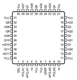
8SLVP1212 40-VFQFPN 6 x 6 x 0.9 mm package body, Top View
