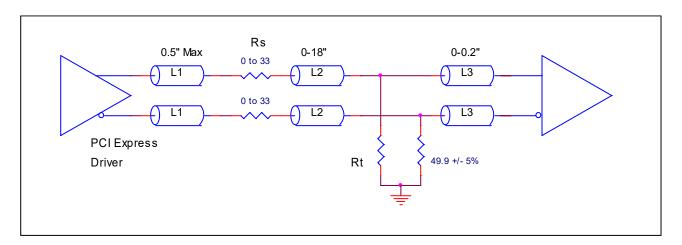
Figure 10B. Recommended Termination (where a point-to-point connection can be used)
