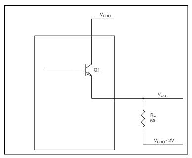
Figure 12. LVPECL Driver Circuit and Termination
