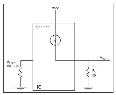
Figure 13. HCSL Driver Circuit and Termination
