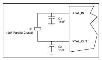
Figure 2. Crystal Input Interface
