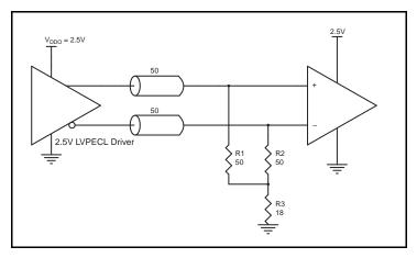
Figure 9B. 2.5V LVPECL Driver Termination Example
