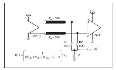
Figure 8A. 3.3V LVPECL Output Termination
