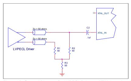
Figure 3B. General Diagram for LVPECL Driver to XTAL Input Interface
