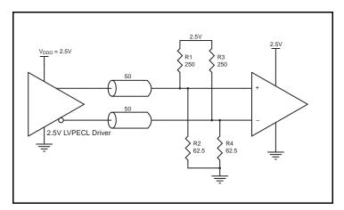
Figure 9A. 2.5V LVPECL Driver Termination Example
