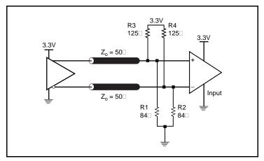
Figure 8B. 3.3V LVPECL Output Termination
