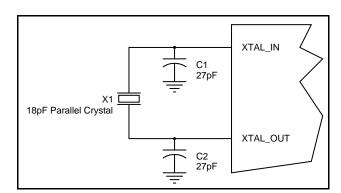
Figure 1. Crystal Input Interface
