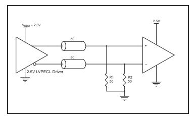
Figure 9C. 2.5V LVPECL Driver Termination Example
