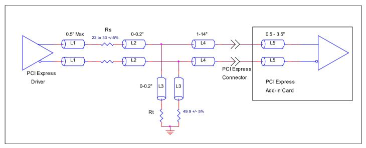
Figure 10A. Recommended Source Termination (where the driver and receiver will be on separate PCBs)
