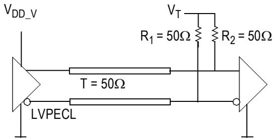
$V_T = V_{DD\_V} - 1.50V$  (250mV Amplitude)
