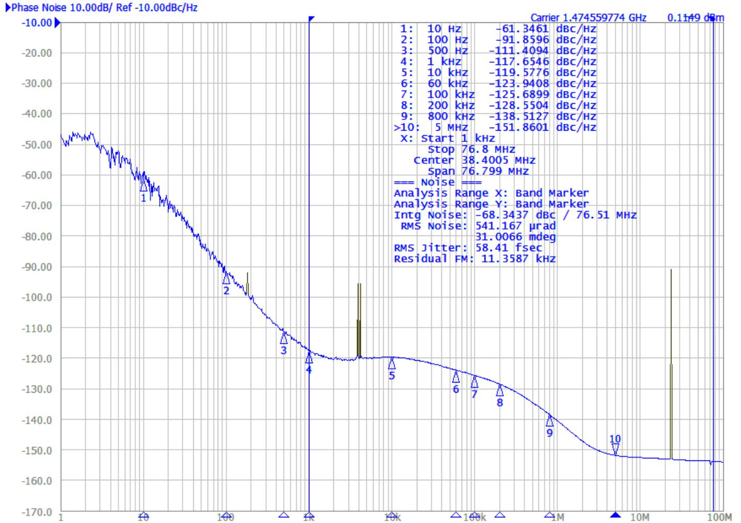
**Figure 10. 983.04MHz Output Phase Noise**
