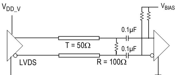
**Figure 15. LVDS (STYLE = 0) AC Output Termination**
