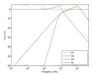
For **PCI Express Gen 2**, two transfer functions are defined with 2 evaluation ranges and the final jitter number is reported in RMS. The two evaluation ranges for PCI Express Gen 2 are 10kHz – 1.5MHz (Low Band) and 1.5MHz – Nyquist (High Band). The plots show the individual transfer functions as well as the overall transfer function Ht.
