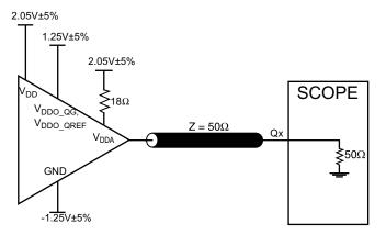
Figure 5. 3.3V Core/3.3V HCSL Output Load Test Circuit 2
