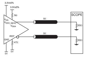
This load condition is used for tjit and odc measurements.
