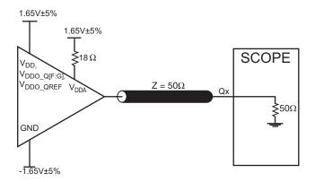
Figure 2. 3.3V Core/3.3V HCSL Output Load Test Circuit 1
