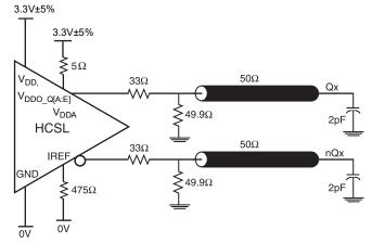
This load condition is used for  $\rm V_{MAX}, \, \rm V_{MIN,} \, \rm V_{RB,} \, t_{STABLE,}$
