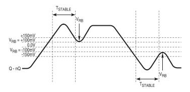
Figure 13. Differential Measurement Points for Duty Cycle/Period
