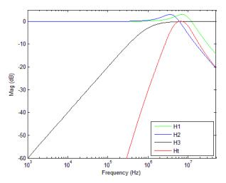
For **PCI Express Gen 3**, one transfer function is defined and the evaluation is performed over the entire spectrum. The transfer function parameters are different from Gen 1 and the jitter result is reported in RMS.
