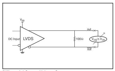
**Differential Output Voltage Setup**
