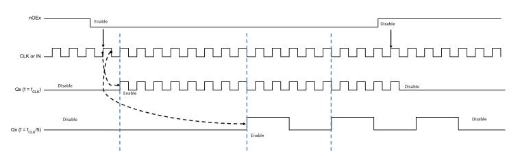
Figure 1. Synchronous Output Enable Timing Diagram
