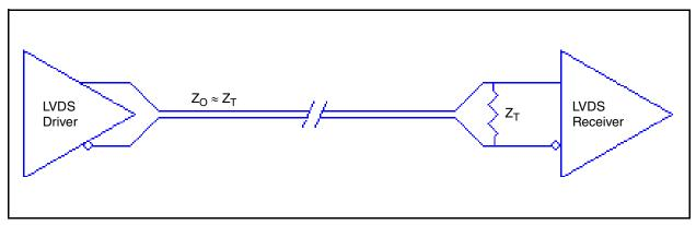
Figure 4A. Standard LVDS Termination
