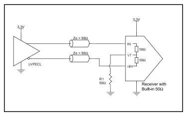
Figure 2B. IN/nIN Input with Built-In 50 $\Omega$  driven by an LVPECL Driver
