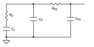
The Rz, Cz and Cp can be calculated as 2<sup>nd</sup> order loop filter. The following equation help determine the 3<sup>rd</sup> order loop filter Rp2 and Cp2.
