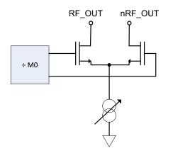
Eight programmable output power levels can be programmed from -4dBm to +7dBm (see RF Output Power).
