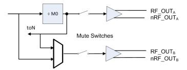
RF\_OUT and nRF\_OUT are derived from the drain of an NMOS differential pair driven by the VCO output (or by the M0 Divider), as shown in Figure 5.
