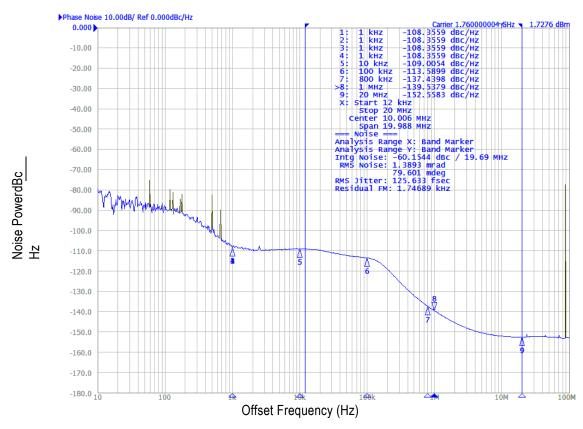
Phase Noise Performance (Open Loop) at 1.1GHz (3.3V)
