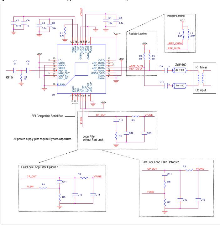
Figure 14. 8V97051A General Application Schematic Example
