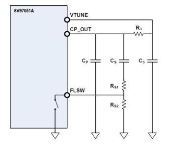
In the example of Figure 9, the damping resistor RS is equal to: RS1 + RS2 in normal mode (FSLW switch OFF), with RS2 = 3 \* RS1
