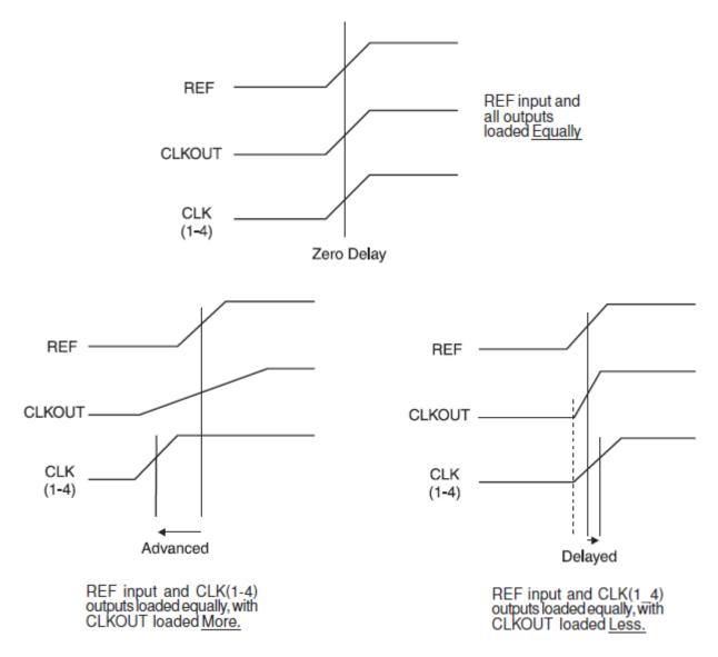
Timing diagrams with different loading configurations
