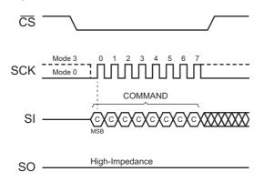
Figure 3. SPI Transfer — Command Only
