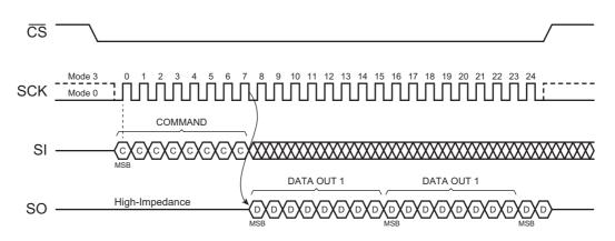
Figure 5. SPI Transfer — Command and Data Only — Read Operation
