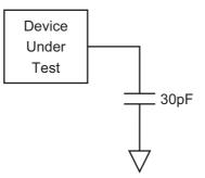
Figure 34. Output Test Load
