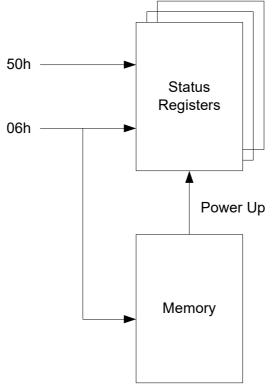
Figure 23. AT25FF041A Register Structure
