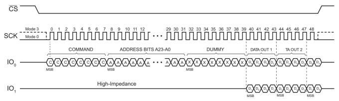
Figure 10. Dual Output Read — 1-Pin Command, 1-Pin Address, and 2-Pin Data
