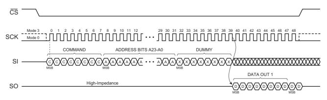
Figure 8. SPI Transfer — Command, Address, and Data — Read Operation with Dummy Bytes
