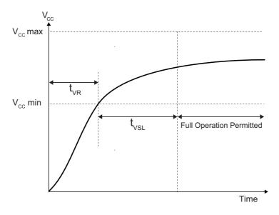
Figure 31. AC Timing During Device Power-Up
