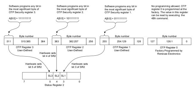
Figure 21. OTP Security Register Program and Lock
