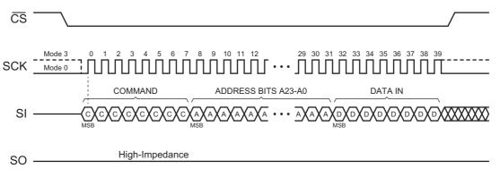
Figure 9. SPI Transfer — Command, Address, and Data — Write Operation
