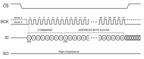
Figure 4. SPI Transfer — Command and Address Only
