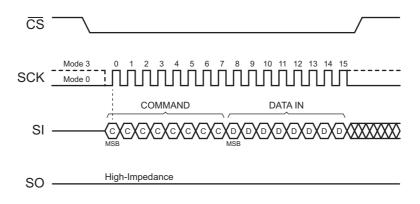
Figure 6. SPI Transfer — Command and Data Only — Write Operation
