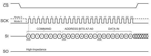
Figure 25. Status Register Write Operation Showing Eight-bit Address Field
