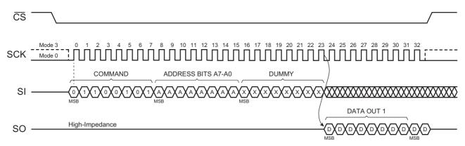
Figure 24. Status Register Read Operation Showing Eight-bit Address Field
