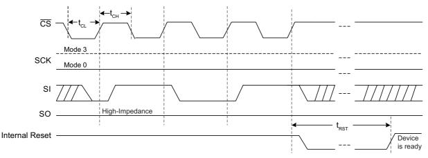
Figure 22. JEDEC Standard Hardware Reset
