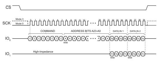
Figure 11. Dual Output Write — 1-Pin Command, 1-Pin Address, and 2-Pin Data
