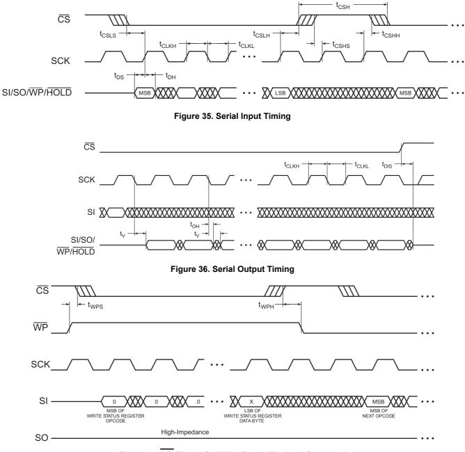
Figure 37. WP Timing for Write Status Register Command
