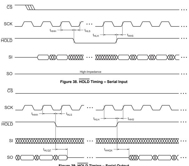
Figure 39. HOLD Timing – Serial Output
