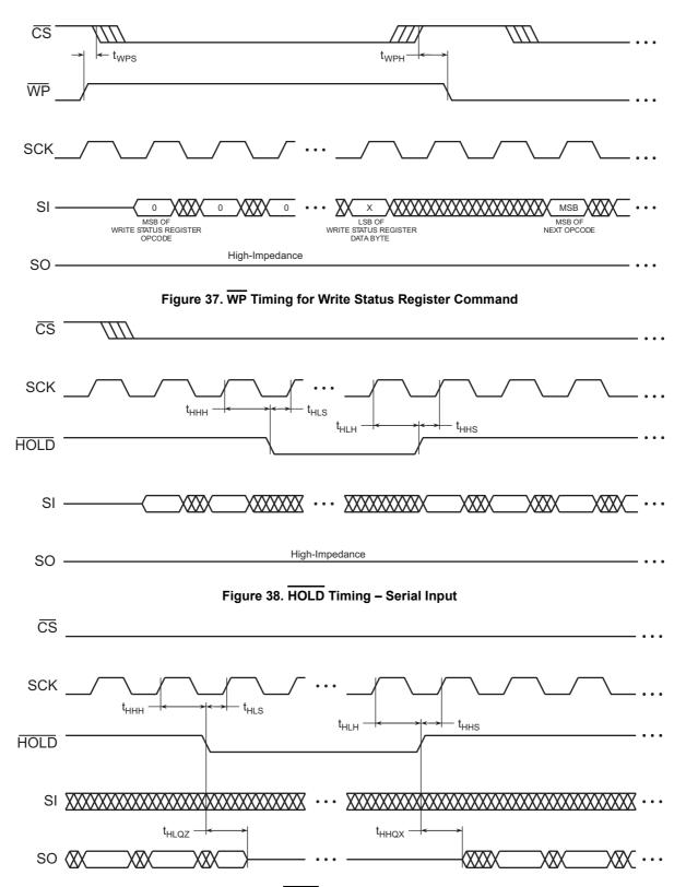
Figure 39. HOLD Timing - Serial Output
