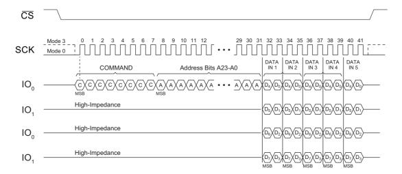
$\textbf{Figure 13. Quad Output Transfer $-$ 1-Pin Command, 1-Pin Address, and 4-Pin Data $-$ Write Operation $-$ 1-Pin Command, 1-Pin Address, and 4-Pin Data $-$ 1-Pin Command, 1-Pin Address, and 1-Pin Data $-$ 1-Pin Command, 1-Pin Data $-$ 1-Pin D$
