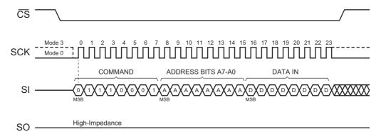
Figure 25. Status Register Write Operation Showing 8-bit Address Field
