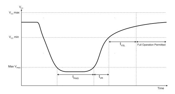
Figure 34. AC Power-up Timing After a Brown-Out
