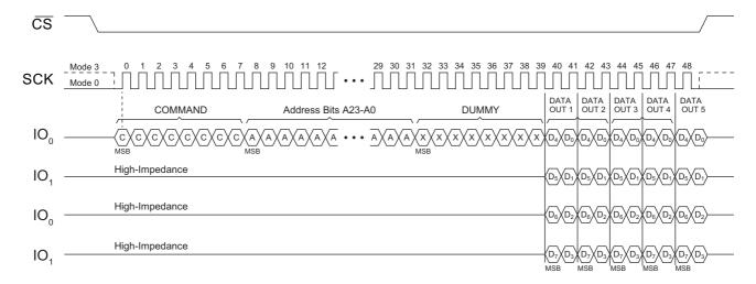
Figure 12. Quad Output Transfer — 1-Pin Command, 1-Pin Address, and 4-Pin Data — Read Operation A 1-1-4 Quad Output write operation is shown in Figure 13. An example of this operation is a *Quad Output Byte/Page Program* (32h).
