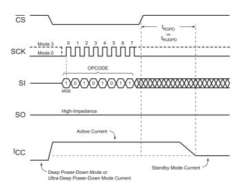
Figure 27. Resume from Deep Power-Down or Ultra-Deep Power-Down
