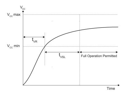
Figure 33. AC Timing During Device Power-Up
