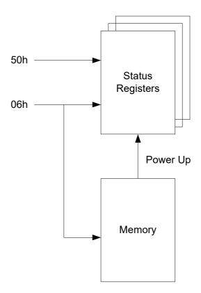
Figure 23. AT25FF161A Register Structure
