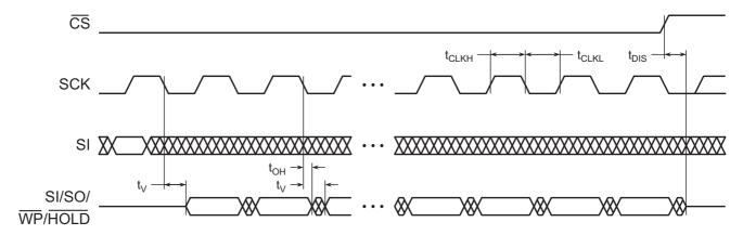
Figure 36. Serial Output Timing
