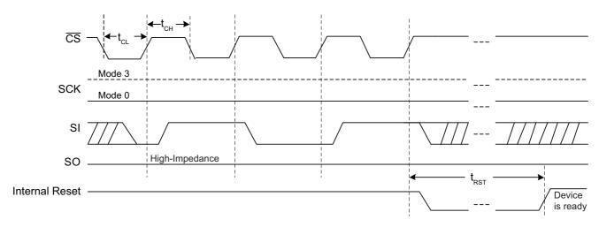
Figure 22. JEDEC Standard Hardware Reset
