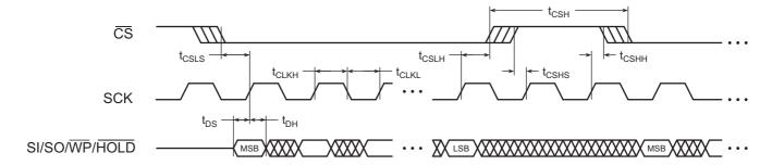
Figure 35. Serial Input Timing
