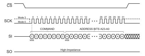
Figure 4. SPI Transfer — Command and Address Only
