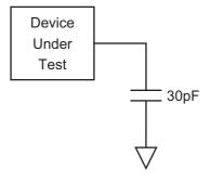
Figure 32. Output Test Load
