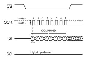
Figure 3. SPI Transfer — Command Only
