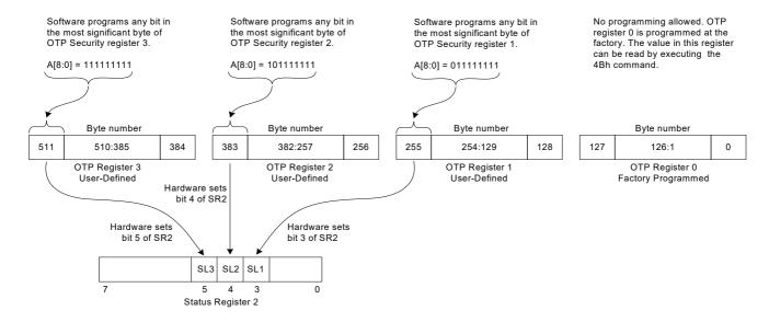
Figure 21. OTP Security Register Program and Lock
