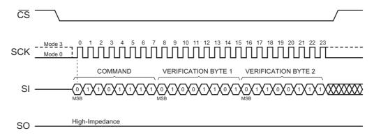
Figure 26. Status Register Lock Operation with Two Verification Bytes
