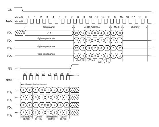
Figure 14. Quad I/O Transfer — 1-Pin Command, 4-Pin Address, and 4-Pin Data — Read Operation
