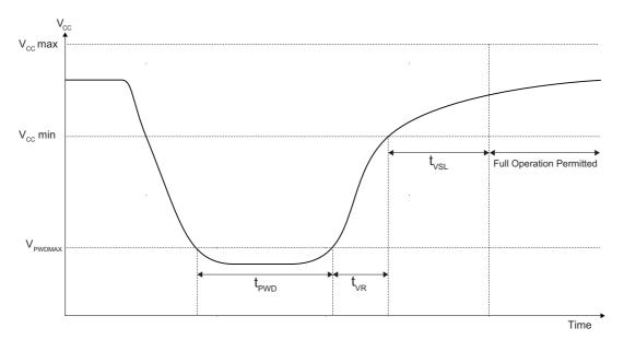
Figure 33. AC Power-up Timing After a Brown-Out
