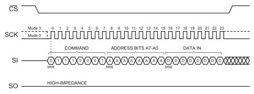
Figure 26. Status Register Write Operation Showing 8-bit Address Field
