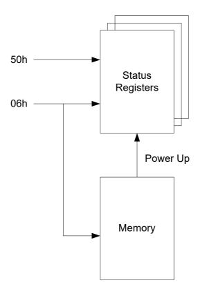
Figure 24. AT25FF321A Register Structure
