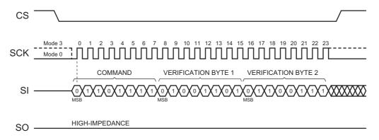
Figure 27. Status Register Lock Operation with Two Verification Bytes
