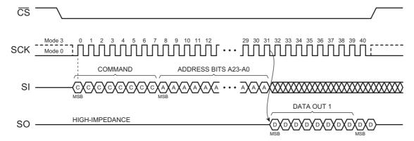
Figure 7. SPI Transfer — Command, Address, and Data — Read Operation with No Dummy Bytes
