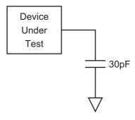
Figure 35. Output Test Load
