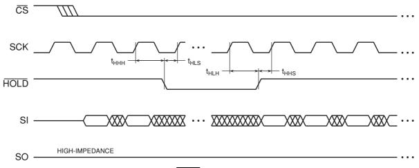
Figure 39. HOLD Timing - Serial Input
