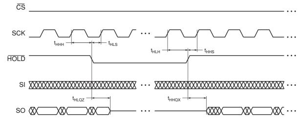
Figure 40. HOLD Timing – Serial Output
