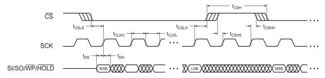
Figure 36. Serial Input Timing
