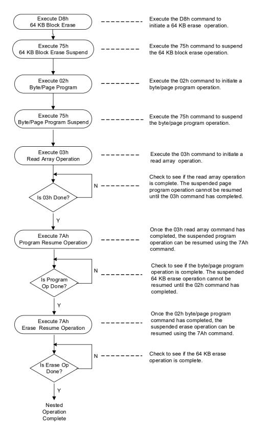
Figure 20. Flow Diagram of Nested Operations Example
