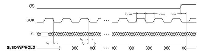
Figure 37. Serial Output Timing
