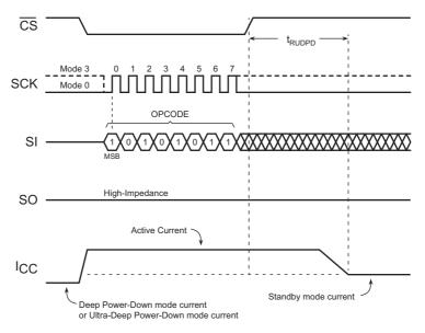
Figure 28. Resume from Deep Power-Down or Ultra-Deep Power-Down
