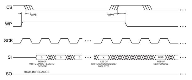
Figure 38. WP Timing for Write Status Register Command
