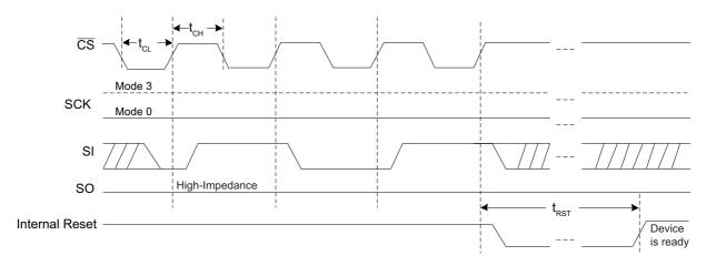
Figure 23. JEDEC Standard Hardware Reset
