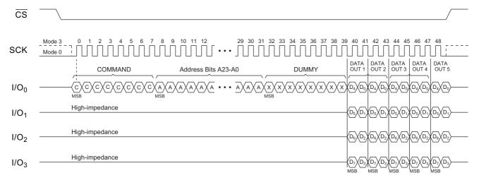
Figure 12. Quad Output Transfer — 1-Pin Command, 1-Pin Address, and 4-Pin Data — Read Operation A 1-1-4 Quad Output write operation is shown in Figure 13.
