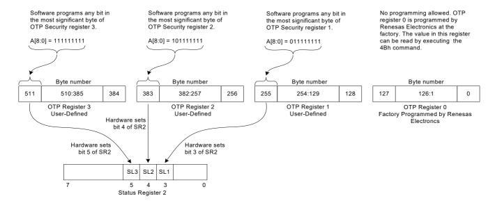
Figure 22. OTP Security Register Program and Lock
