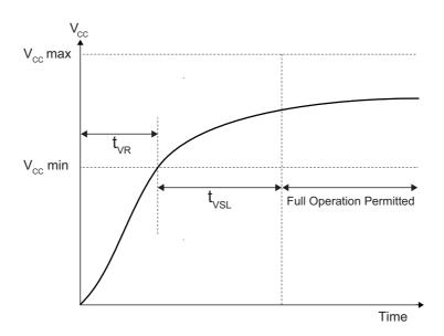
Figure 32. AC Timing During Device Power-Up
