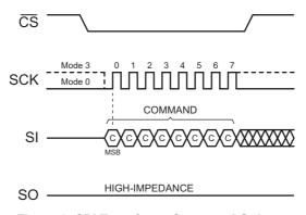
Figure 3. SPI Transfer — Command Only
