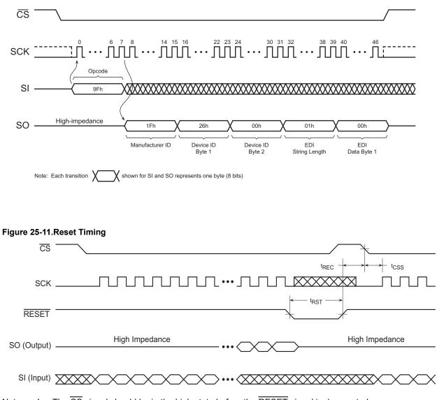
Note: 1. The CS signal should be in the high state before the RESET signal is deasserted.
