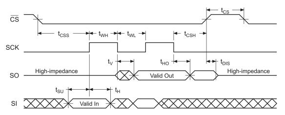
Figure 22-1. Waveform 1 = SPI Mode 0 Compatible
